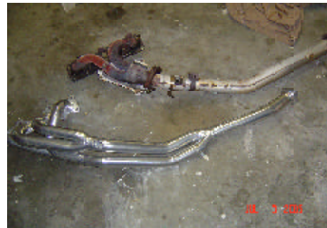
Jackson Racing's header next to a stock '94 header. Quite a difference!
